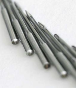
Using sewing needle diameters that are too large on thin leather materials creates unnecessarily large puncture holes. These can weaken the leather seam or even cause the seam to tear. However, if a needle size that is too small is used for the sewing thread, the thread material may bunch up or even break.
