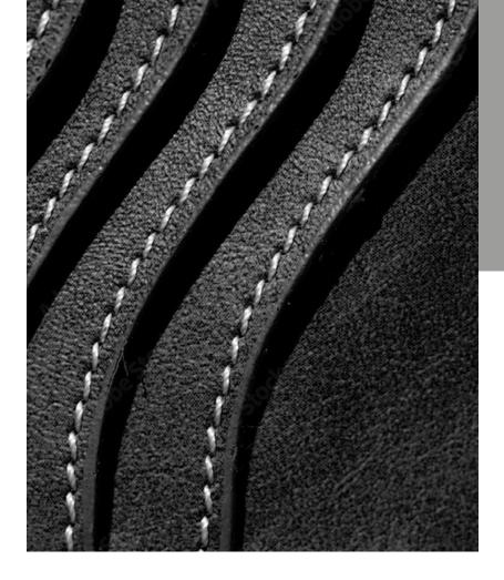
Eye-catching seams are often used as a special design element. In particular, these are achieved with coarser sewing threads with a round thread cross-section.
