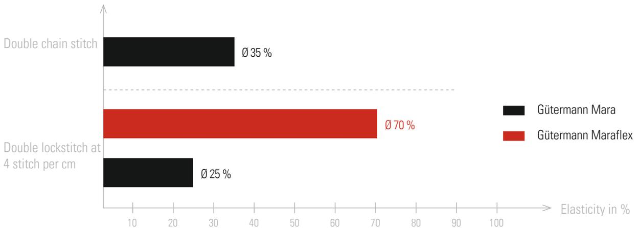
Maraflex was specifically developed for the use on both lockstitch and chain stitch machines when stitching highly elastic fabrics. Maraflex is the reliable partner when it comes to lockstitch
